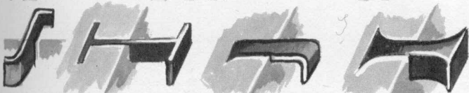
METAL CRAMPS set in molten lead
